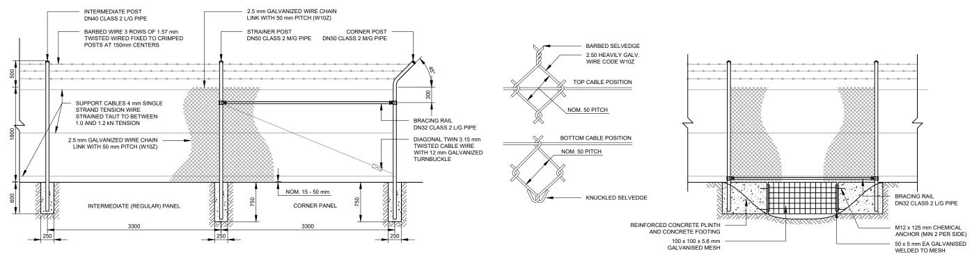
FENCE AND GATES TO BE DESIGNED AND CONSTRUCTED TO AS 1725 PART 1
